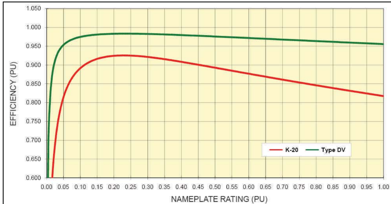
Graph #2 - Comparison of Non-Linear Load Operating Efficiency 75kVA K20 Rated Transformer vs. 75kVA PQI “DV” Type HMT Transformer
